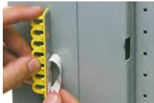
2. Attach the lockout device to the breaker and snap into locked position
