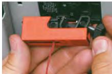
3. Pass plastic key through lock rail and attach lock, preventing key from sliding down cable and opening lockout device
