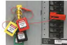
5. Low-profile lockouts allow panel doors to be closed on most breaker panels.
