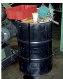
No more pump drips sliding down the side of the drum and onto the floor.
