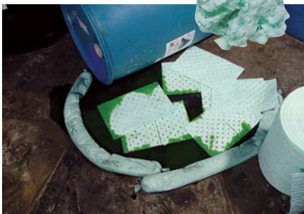
Fast containment of chemical spills.
