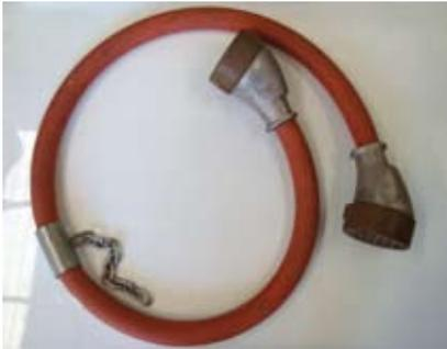
XPT and MU Locomotive Jumper Cables
