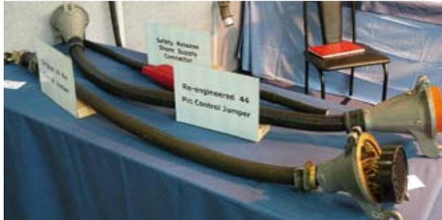
Old and New Style 44 Pin Communication Jumper Cables
