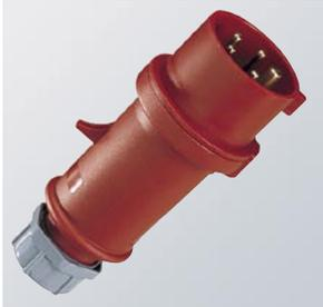
⚠ IP 44 plug **StarTOP®** with screwless insulation piercing technology **SafeCONTACT**. Gland with grommet, strain relief, and cable kink protection, enclosure with thread lock and safety slide.
