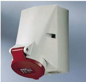
▲ IP 44 wall-mounted receptacle, fastening from inside, entries - one on top and two blind (to cut out) at the bottom, lower part of housing can be rotated 180° screwless spring terminal technology **TwinCONTACT**, connecting terminals suitable for through wiring.
