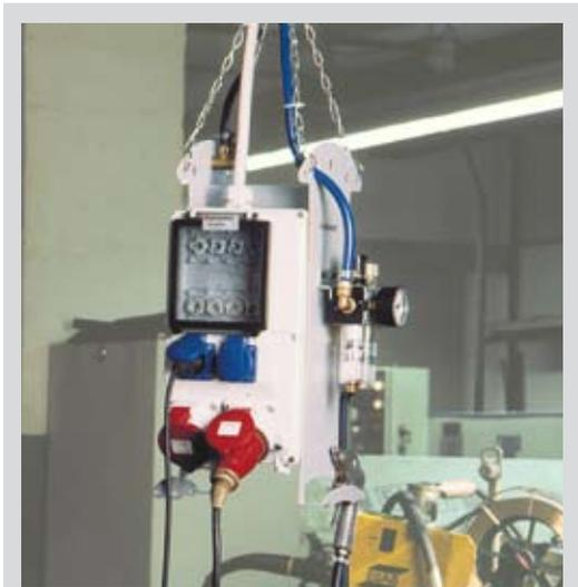
The swift, value for money concept for individual pieces of equipment using receptacle combinations and compressed air ports
