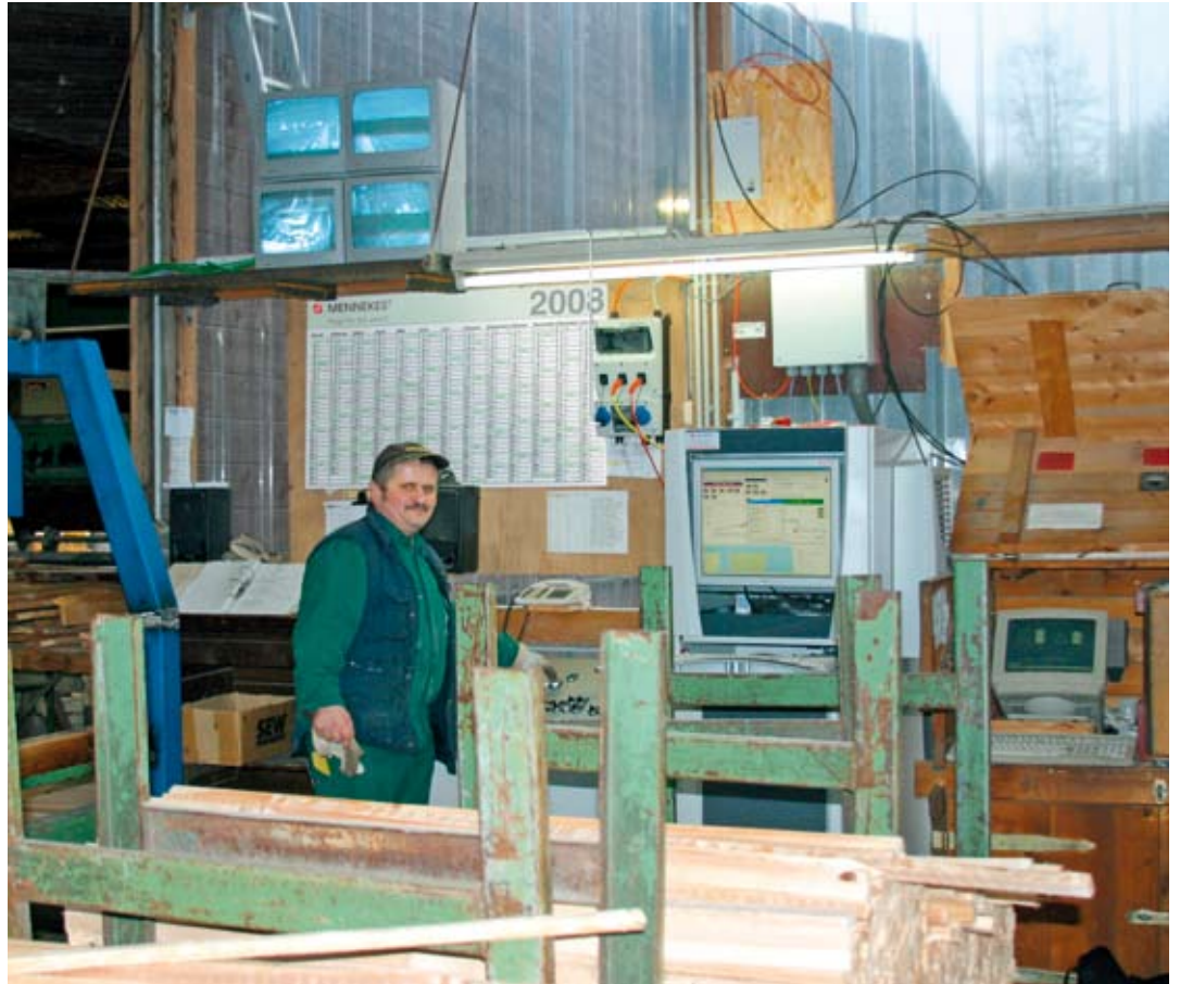
AMAXX network enclosure for safe installation in dusty areas.
